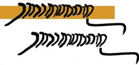
This involves tightly winding wire around small pipe to create a spring.
